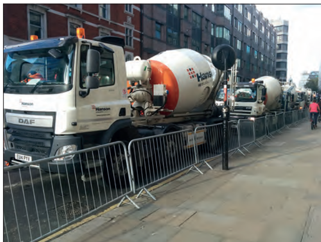
Figure 1. Concrete lorries in the lorry holding area at the Moorgate shaft site – the logistics team had to manage 800 hauliers delivering to approximately 30 main contractors across more than 50 central London sites
