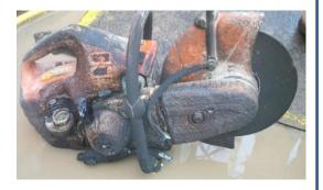
On 6<sup>th</sup> March a small fire occurred when a piece of material ignited after being showered in sparks from a stihl saw which was being used to cut steel. The fire was extinguished immediately.
