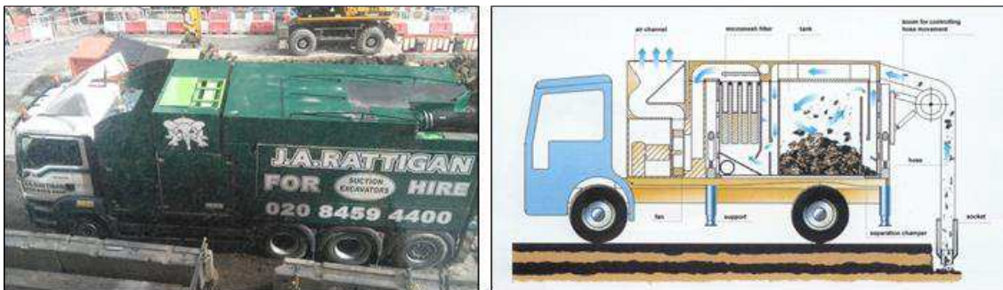
Fig. 15 – Left: vacuum excavator at Liverpool Street (Copyright Crossrail Ltd); Right: diagram of vacuum excavation equipment (Courtesy of SUC-EXC UK LTD)
