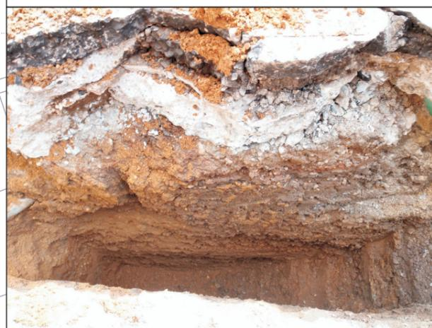
Plate 2: Test trench at the northern end of trench 4 showing river gravels overlain by modern made ground
