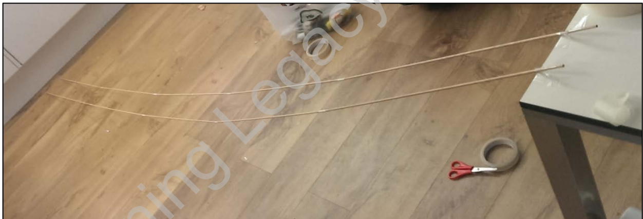
Fig A: Rail sloping from table to floor. Sloping to floor will ensure that rail cars do not derail at the end and break. Notice that the top of the rail is at a slope, not parallel with the table.
