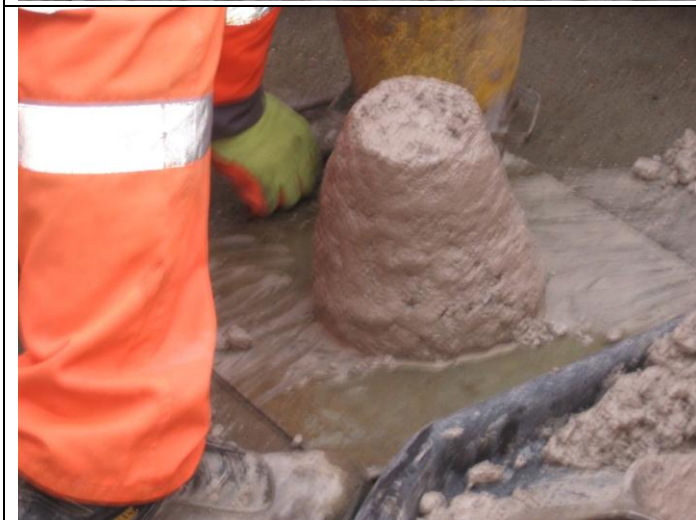
Photograph 18 Second Block Trial, slump prior to pouring 21st November 2013
