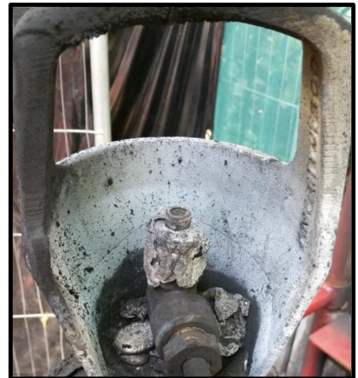
Top of a badly burned acetylene cylinder
