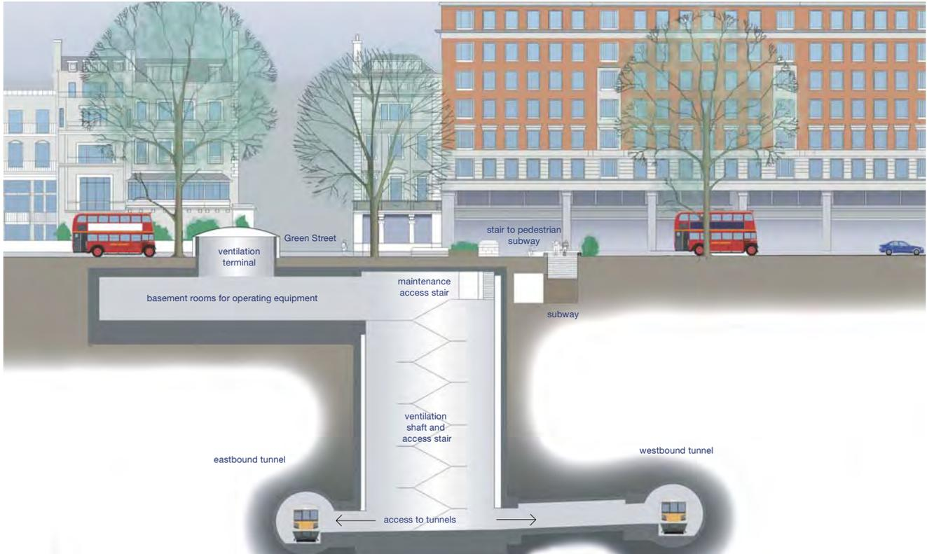
Section Through Ventilation Shaft Looking East
