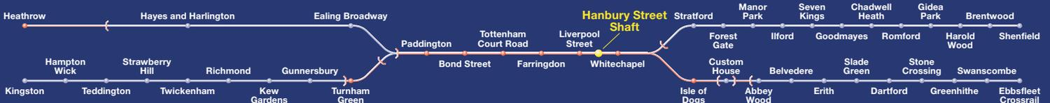
The shaft is proposed to be located at the junction of Hanbury Street and Princelet Street and would provide emergency access and ventilation to the Crossrail tunnels between Liverpool Street and Whitechapel Stations.
