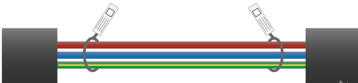
Figure 6: Multicore cables cable-tied to form one asset
