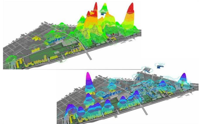
Figure 7: Analysis and Visualisation of Footfall within a Facility
