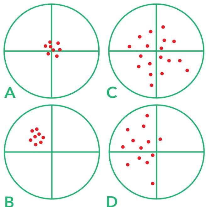
Figure 11: Accuracy vs Precision
