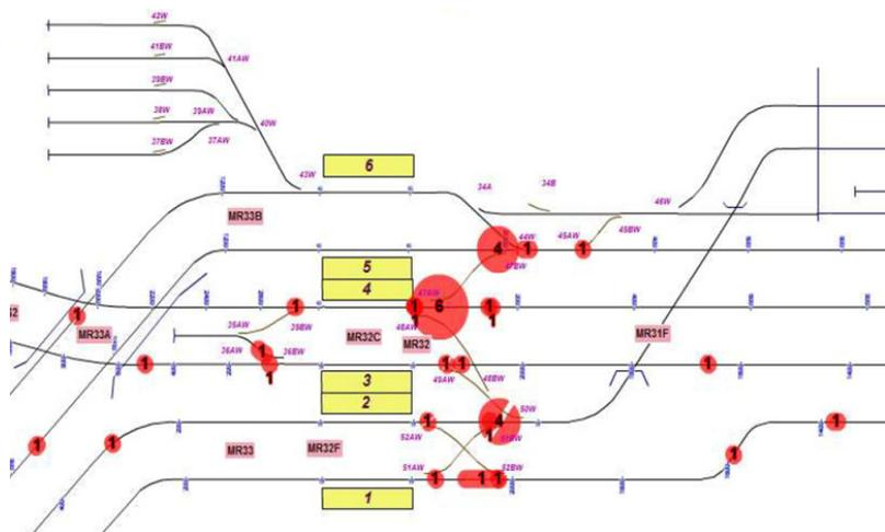
Figure 5: Cluster Analysis of Work Orders on Operational Railway
