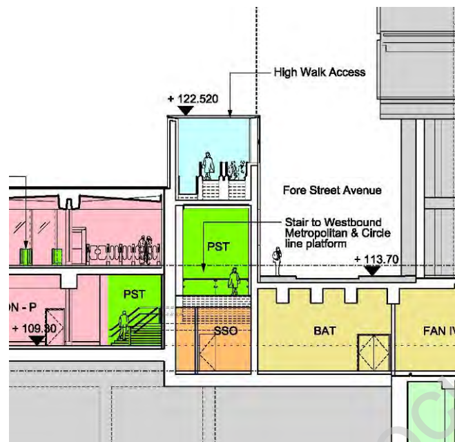
Figure 3-1: Diagram illustrating how the WB stair is constructed below the CoL Highwalk Escalators
