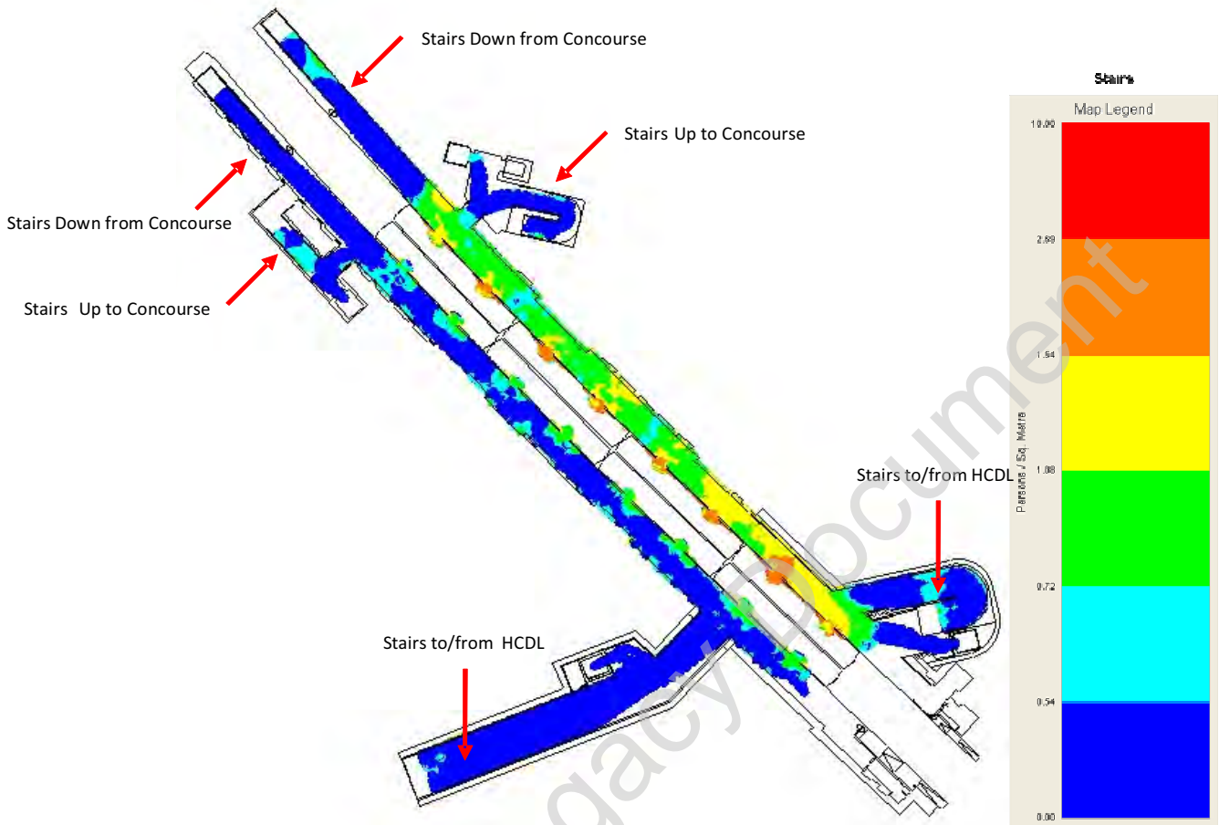
Figure 6.14 – Level of Service (CMD Stairs) – 2026 +28% PM Peak 15 Minutes
