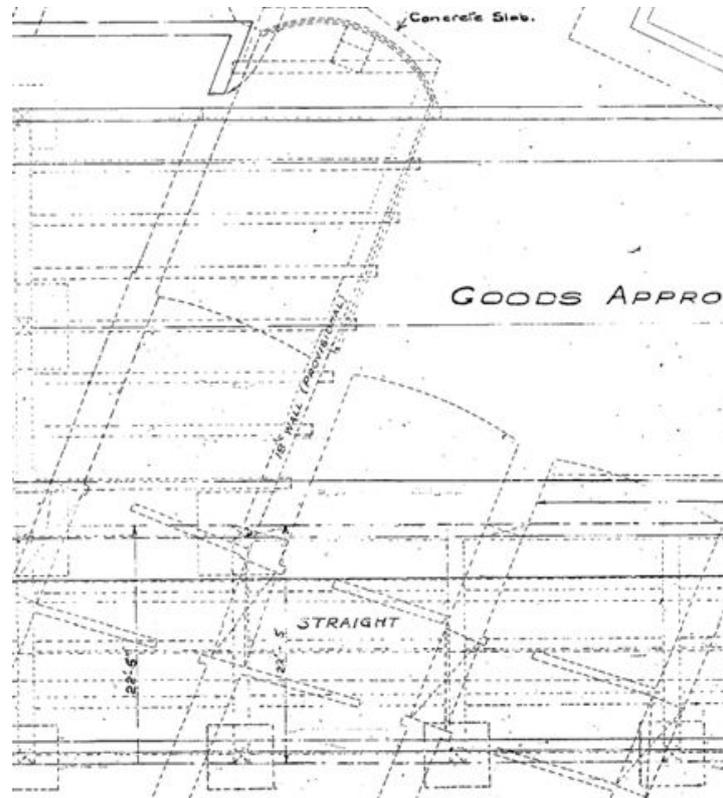
**Figure 14 - Full extent of vault 7 seen here are 8 and 9 to the right. Note access to the south route that divided (source: G.W.R Paddington Station Improvements: Bishops Road Station, Goods and Taxi Approach Roads. General Plan of Reinforced Concrete Work, Contract No. 11, Drawing No. 2)**
