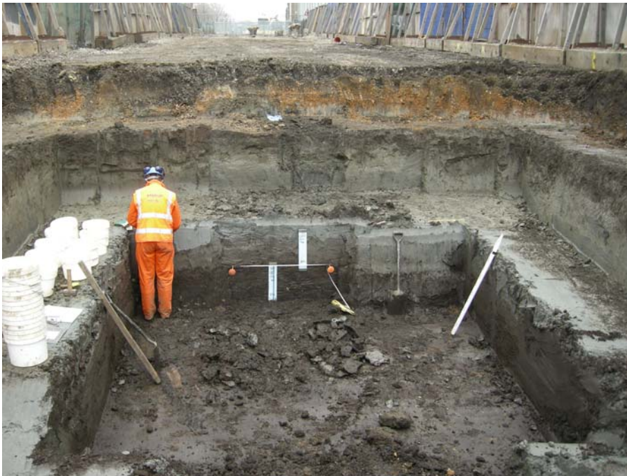
Photo 4, Looking east, sampling of transition between upper clay and lower peats.
