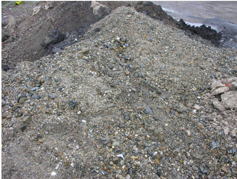
Photo 7 Natural gravel from the base of Drive Pit SL6a
