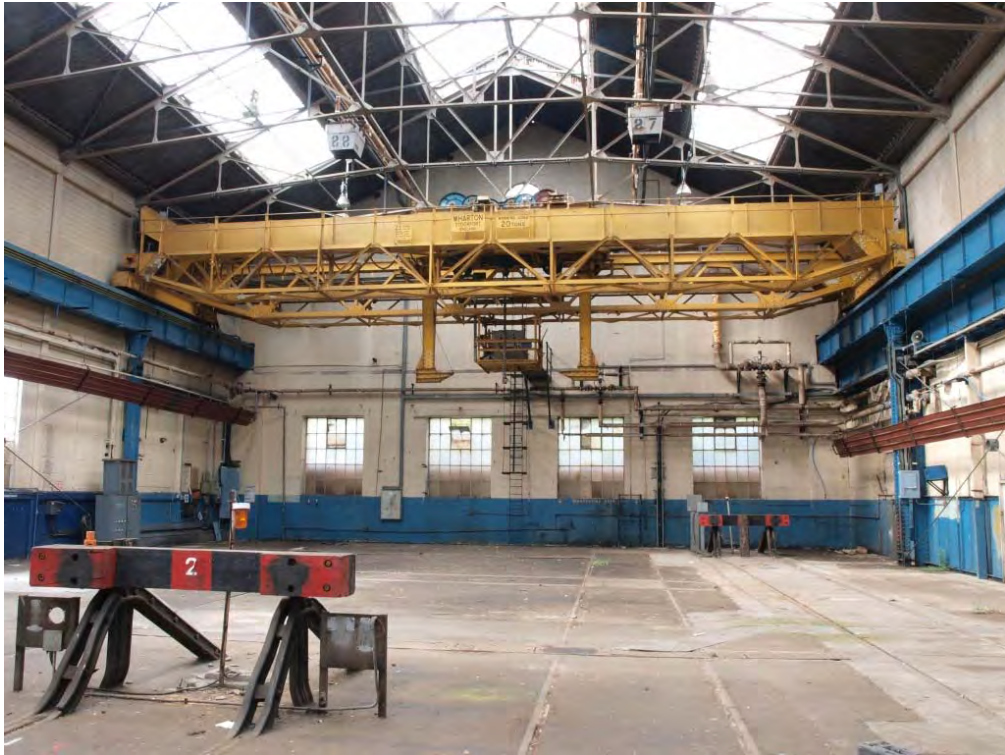
Plate 63. Wharton gantry crane at west end of Carriage Lifting Shop (23)
