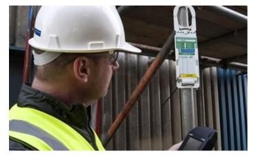
Tags. RFID tags use radio waves to communicate with the digital receiver used during inspections and are completely passive, meaning that they do not require batteries or a power source to operate. RFID is recommended for use in rugged industrial environments. A variety of Tags are available that are resilient to wear, water, dirt, chemicals, etc.
