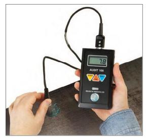
The Audit 106 has 10 preset calibrations to measure, amongst others, mild steel, stainless steel, aluminium, copper and iron ranging in thickness from 1.5mm to 99.9mm, with a sensitivity of 0.1mm. The Audit 106 unit contains a 6mm test block on the front panel which serves as a confidence check to ensure the correct operation of the instrument and probe.
