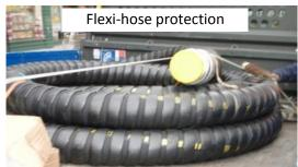
2) Protection of hoses from site traffic. Some examples are shown below, however the overall outcome should be the prevention of contact between vehicle traffic and hoses (whether under pressure or not), minimising risk of damage.
