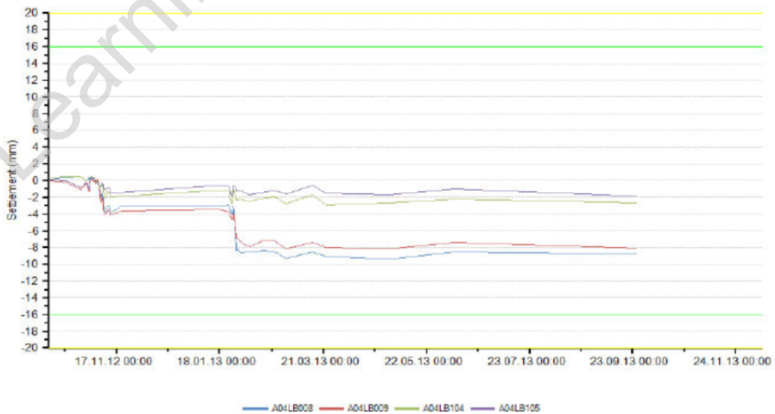
Figure 17: data time-plots - comparison against settlement triggers
