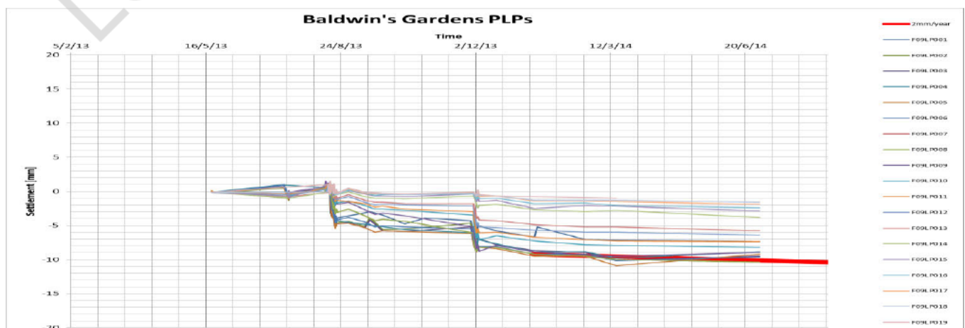
Figure 26: data time-plots - comparison against 2mm/year settlement rate (long-term)
