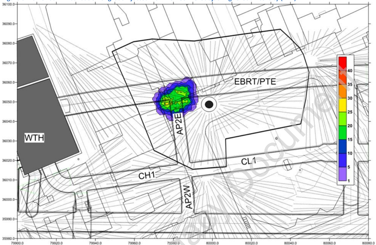
Figure 3.7.3 Period F: Distribution of grout injected from TCR GS2: Grout jacking. Grout Intensity (mm).
