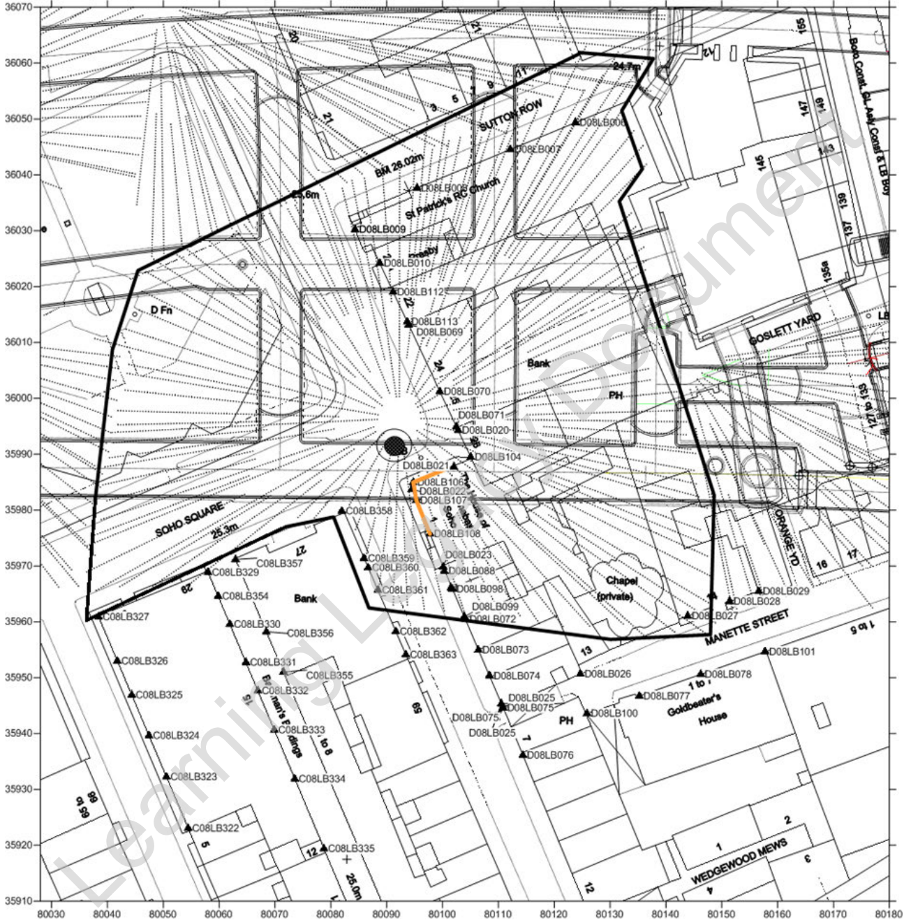
Figure 4.1. Locations of BRE and building slope Amber trigger breaches.
