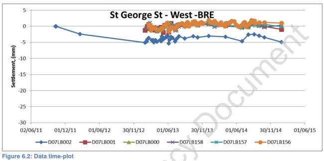
The points on the façade on the west side of St. George Street show negligible impact (<5mm) from C300 works. The overall long term rate of settlement is less than 2mm/year. The residual risk associated with long-term settlements is considered to be negligible.
