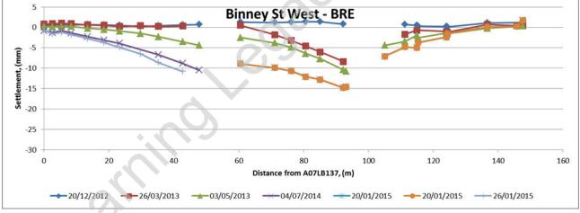
Figure 2.7: Profile plot: Binney Street West facade
