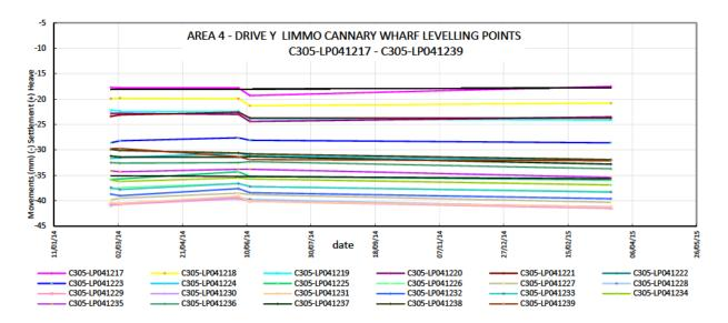
The graphs and tables of settlement rate for both transects show that settlement rate due to dewatering works is less than 2 mm/year. As the instruments in this report are located between these two transects it is concluded that they will behave in a similar manner and hence their settlement rate will be less than the 2 mm/year rate.
