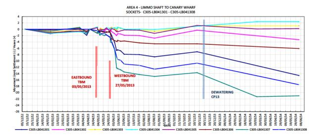
The graph above shows a maximum settlement of -2 mm during the Eastbound TBM transit and an additional -12 mm settlement during the Westbound TBM transit for the socket C305-LB041307.
