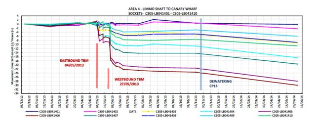
The graph above shows a maximum settlement of -9 mm (C305-LB041405) during the Eastbound TBM transit and an additional -13 mm settlement (C305-LB041406) during the Westbound TBM transit.
