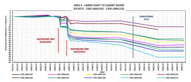
The graph above shows a maximum settlement of -11 mm (C305-LB041210) during the Eastbound TBM transit and an additional -15 mm settlement (C305-LB041209) during the Westbound TBM transit.
