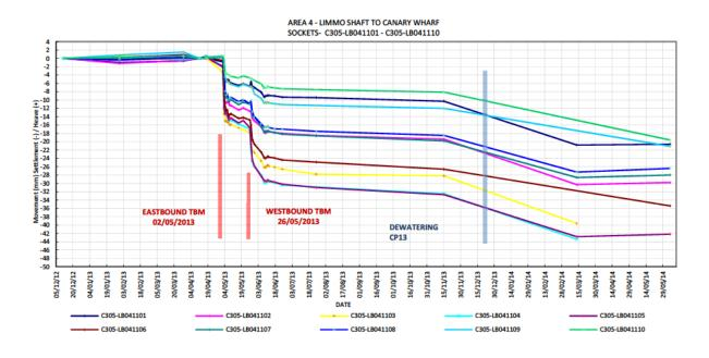
The graph above shows a maximum settlement of -16 mm during the Eastbound TBM transit and a -14 mm settlement (C305-LB041104 and C305-LB041105) from the Westbound TBM transit.
