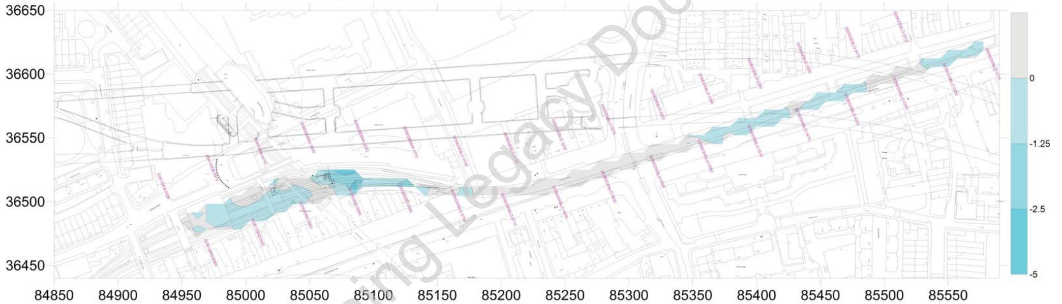
Differential Movement Z (mm) from 30/10/2014 to 30/04/2015 - Track and Structure
