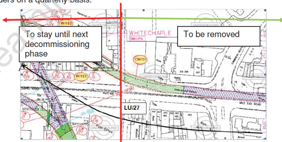
Figure 1 - LU District line Assets included in interface LU/27 are highlighted in yellow (Extract from Metronet Drawing NNNN0000-DWG-CVL-SA00-5531234, Rev 02)
