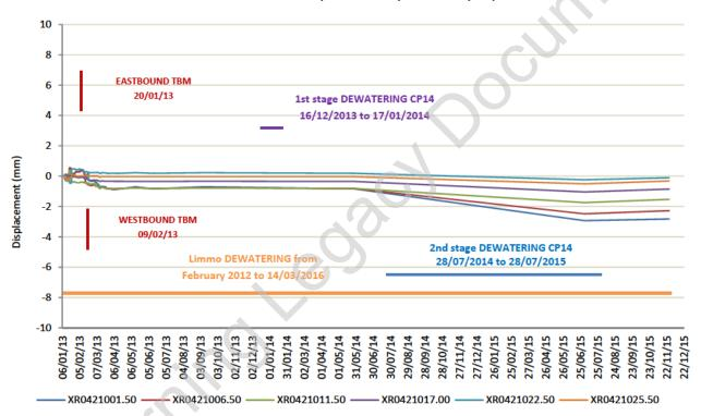
The graph presented below shows the readings from this rod extensometer, showing a maximum total settlement of 0.70 mm during the Westbound TBM transit. A maximum of 15.88 mm of settlement was recorded in November of 2015.
