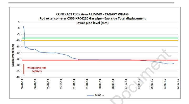
The graph presented below shows the readings from this rod extensometer, showing absolute differential displacement of both pipe levels. Absolute maximum displacement value of 4.92 mm was recorded in November of 2015.
