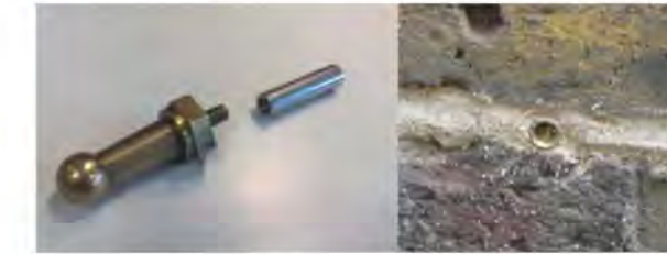
BRE Levelling Stud: Levelling stud screws into BRE socket within wall. Manually read levelling staff placed onto stud.
