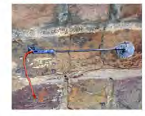
Vibrating Wire Crackmeter: Vibrating Wire Crackmeters measure the expansion and contraction across existing cracks and joints. They are read from a transmitter box located on the façade.
