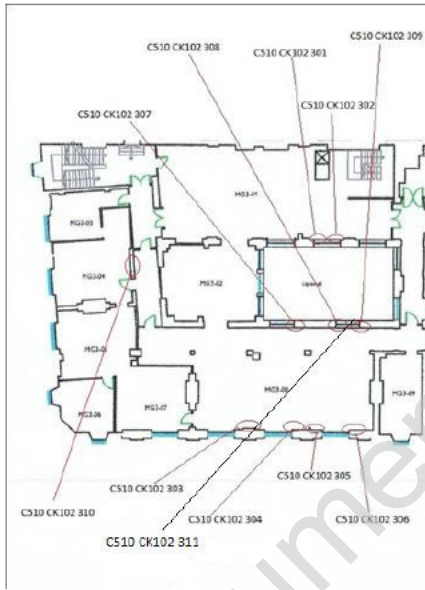
Crackmeter Location Plan 3rd Floor
